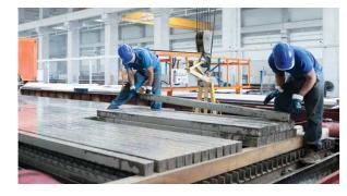
End pole orcharding Section 1: 95 x 95 mm Section 2: 100 x 120 mm
